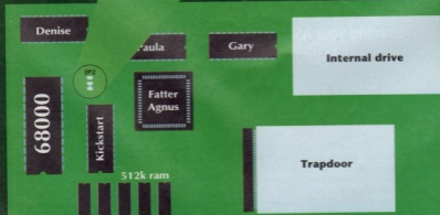
This is the solder job you'll be faced with if you decide to upgrade the A500 to one meg of chip ram
